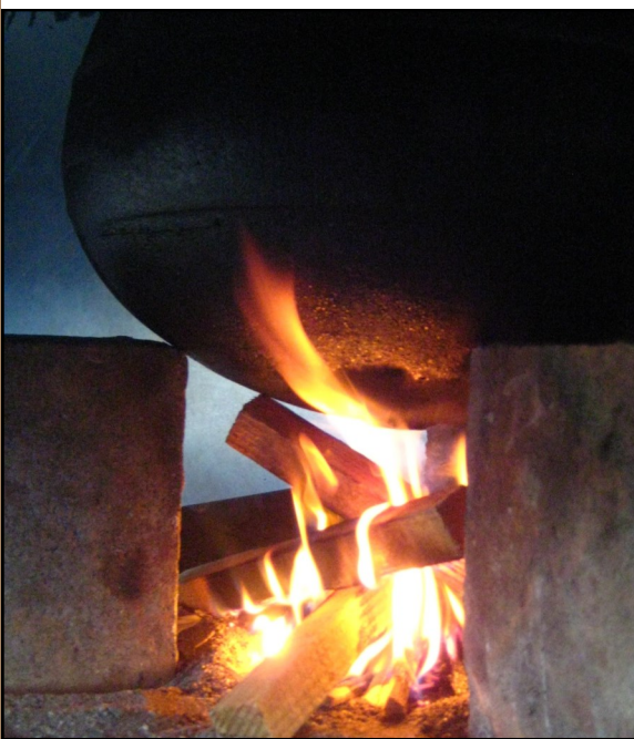
Figure 1. Photo of a traditional three stone fire. During each wood-burning experiment, wood is continually added to the fire to heat 2kg of water from room temperature to boil. The orange hue of the flame front is indicative of the production of black carbon (or soot) particulates emitted in the ultra-fine particle size mode (<100nm in diameter).
